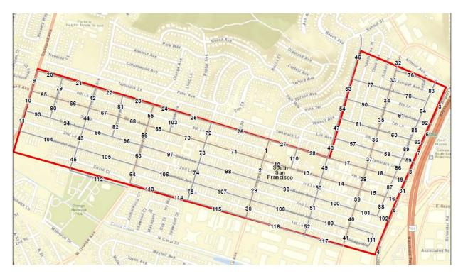
SmartWAVE will install 105 Wi-Fi access points, and wireless backhaul equipment on PG&E and City poles with internet speeds capable of 100Mbps symmetrical download and upload. The network will extend 117 city blocks and provide internet service of 10Mb symmetrical speeds to over 12,000 residents in the area. This Wi-Fi service will provide basic internet access which can be used for virtual meetings, online classes, and career resources for job seekers.
