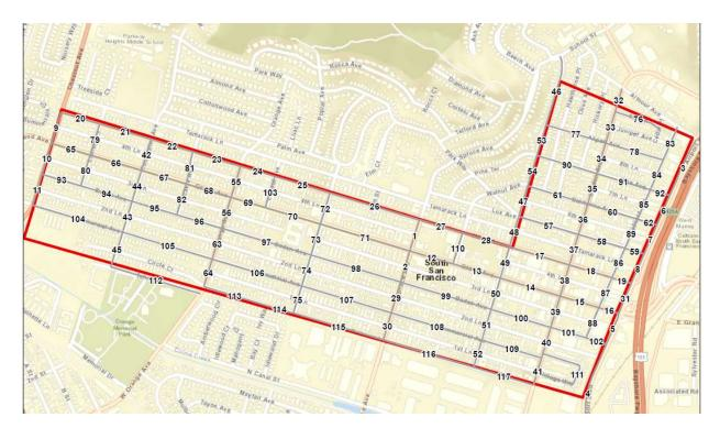
SmartWAVE will install 105 Wi-Fi access points, and wireless backhaul equipment on PG&E and City poles with internet speeds capable of 100Mbps symmetrical download and upload. The network will extend 117 city blocks and provide internet service of 10Mb symmetrical speeds to over 12,000 residents in the area. This Wi-Fi service will provide basic internet access which can be used for virtual meetings, online classes, and career
