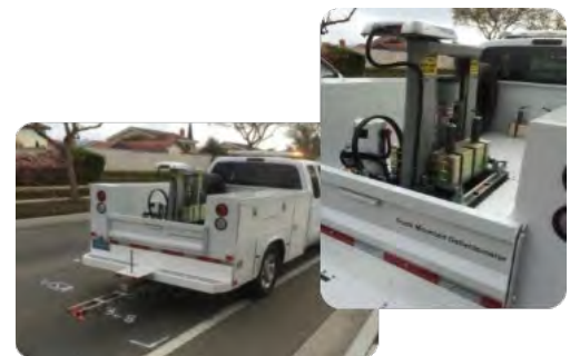
Figure 8 – Falling Weight Deflectometer Testing
