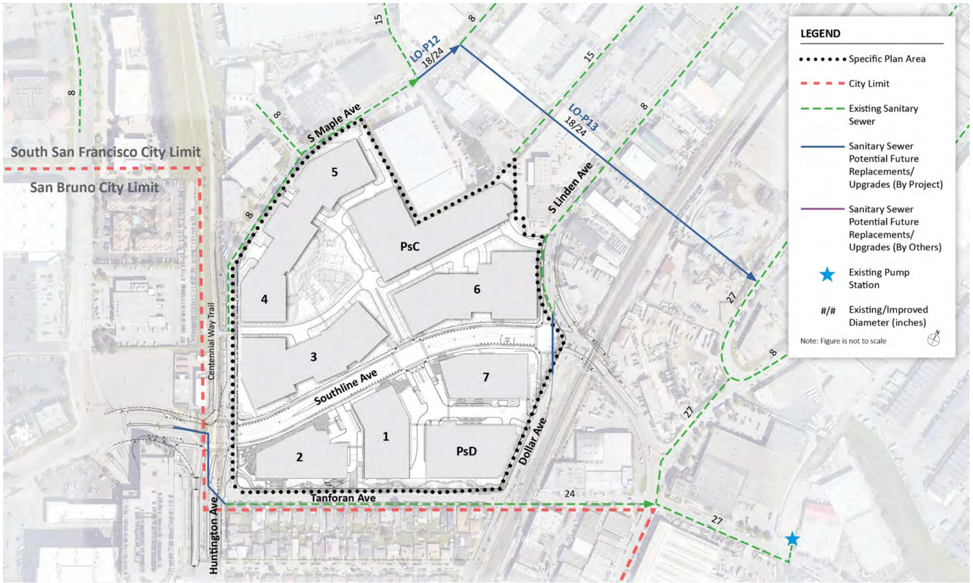
Figure 4-2: Conceptual Wastewater Improvement Plan
