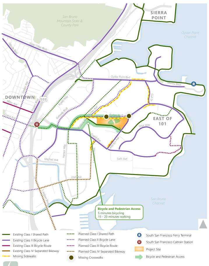
Figure 2-2 Existing and Planned Bicycle and Pedestrian Facilities
