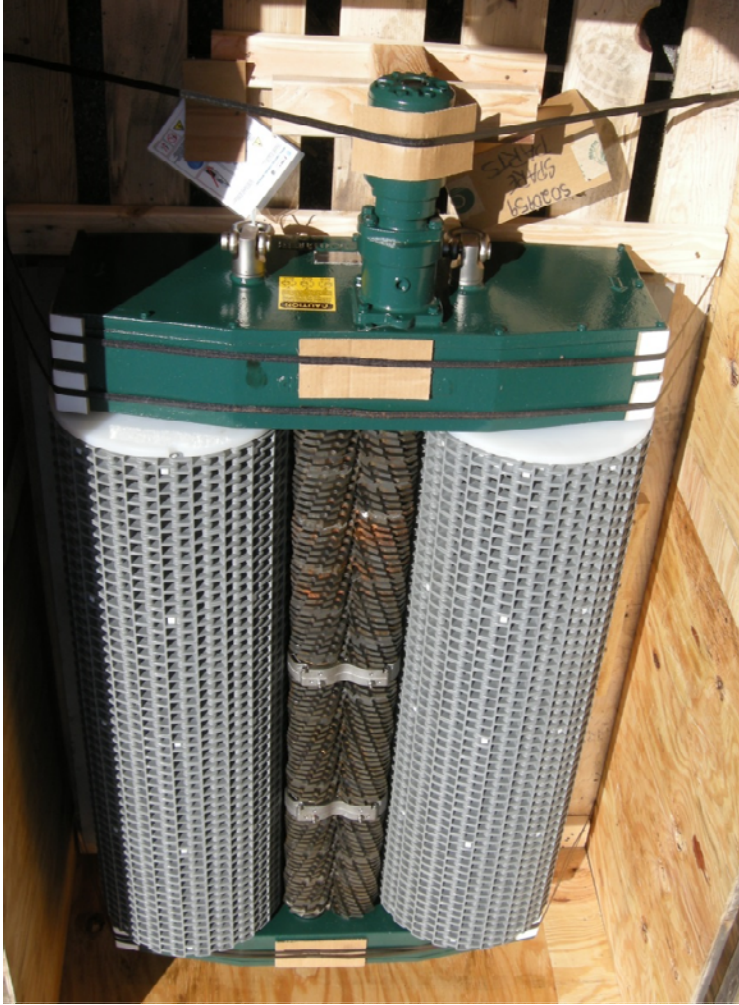
Sewage Grinder After Refurbishment
